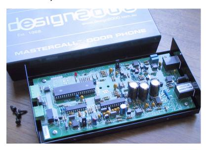
① Locate LK2 - the three pin "US\_AUS" jumper link circled below in red:
