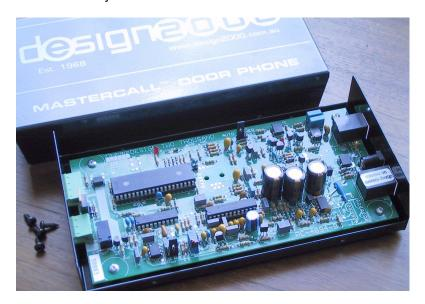
① Locate LK2 - the three pin "US\_AUS" jumper link circled below in red:
